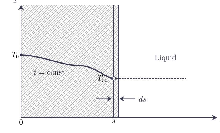
Temperature profile (for t = constant) for the solidifying of a plane solid. s is the distance between the phase boundary and the cooled surface x = 0.
