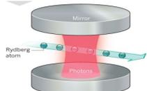
Rydberg atoms, which have one electron in a high-energy level, are sent through the system to measure and manipulate the photon's quantum state.
