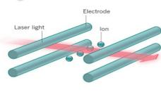
Laser light is shone on the ion, suppressing its thermal vibration and allowing its quantum state to be measured and controlled.
