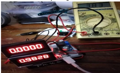
Photo of the circuit used in lithium-ion battery current measurements.
