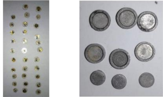
Fig.2 Sample holders that are inserted into the channels, gold dics and cover cadmium
