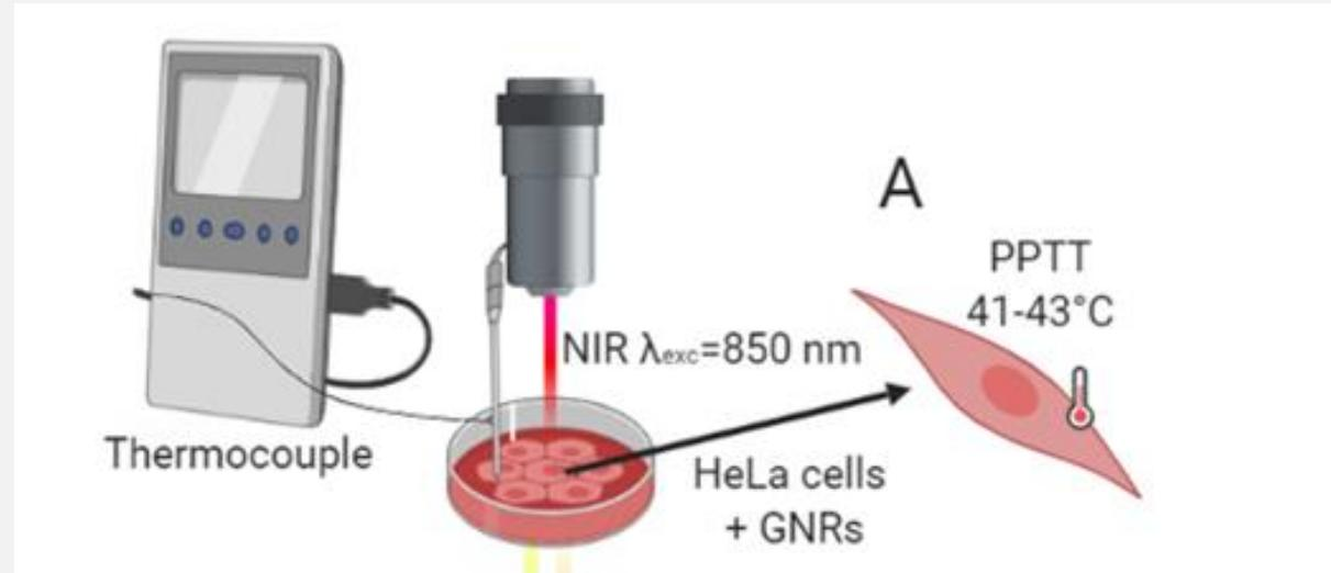
The microscope includes an optical fibre, an 850 nm laser was coupled to this fibre and the IR light was delivered directly into the microscope objective to the sample.
